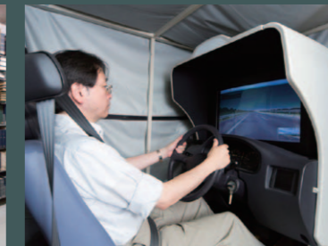
Car driving simulator for measuring how fatigue affects drivers
